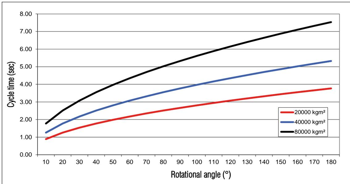
\* Please note, the load chart shown can be affected by user programming required, including acceleration rates, deceleration rates, velocity profiles, e-stop times required, etc. For validation of sizing, please verify all loading with Motion Index Drives, Inc.
