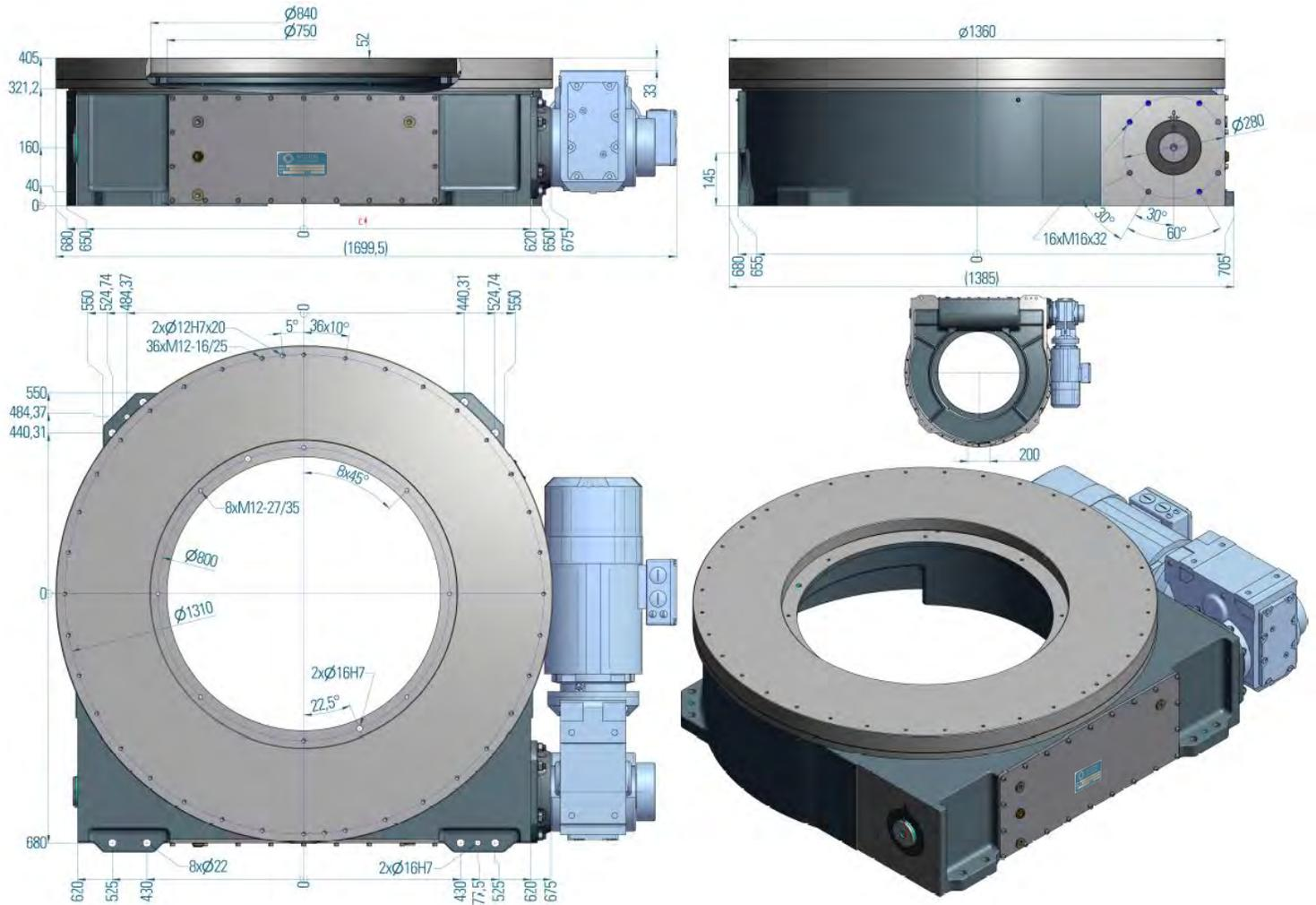
**!** The dimensions for the gearmotor may change based on the gearmotor size and options required for the application.
