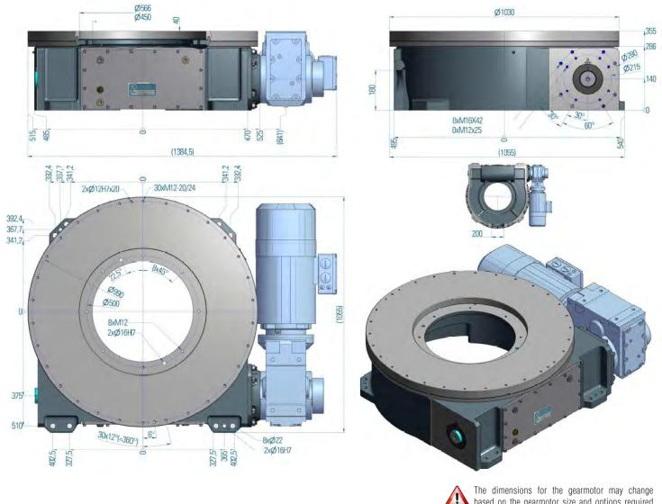
The dimensions for the gearmotor may change based on the gearmotor size and options required for the application.
