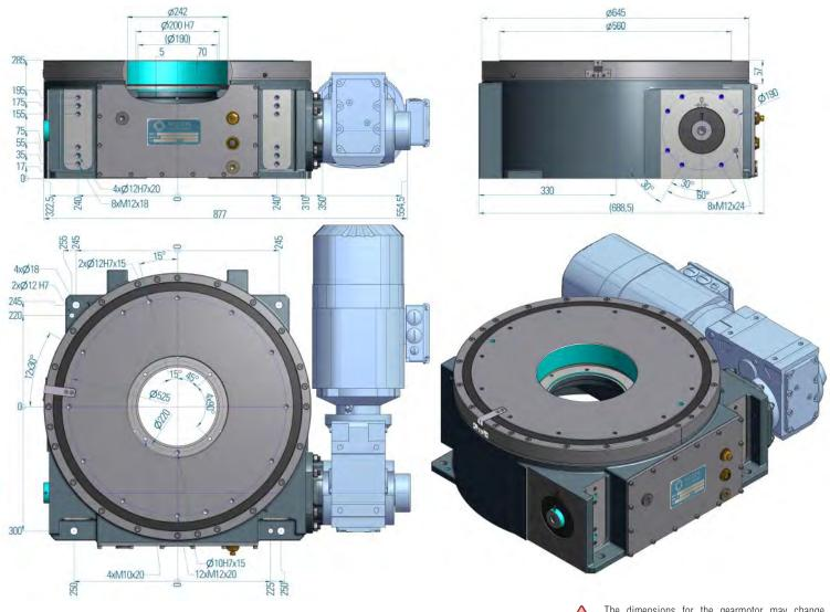
The dimensions for the gearmotor may change based on the gearmotor size and options required for the application.
